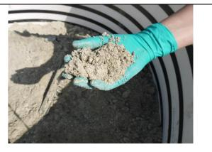
Gypsum and moraine mixed and compacted in the lysimeter vessel.
