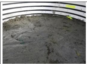
Fine tailings sand compacted in the lysimeter vessel.
