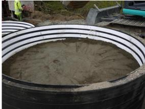
Tailings sand + 10 % ash mixed and compacted in the lysimeter vessel. Figure 7. Field tests in Pyhäsalmi mine in 2016.
