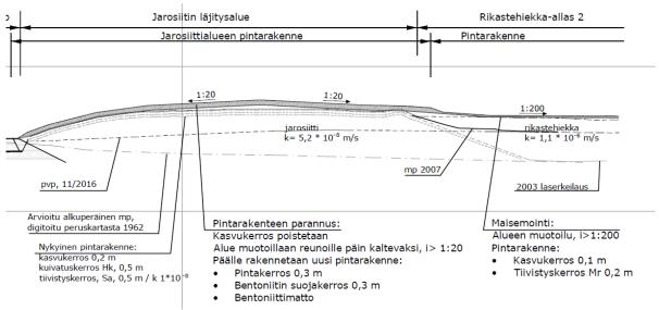
Figure 9. The initial plan was to use 0,20 m layer of moraine on top of tailings sand (on right the side of picture), which was substituted with 0,25 m fiber clay layer.
