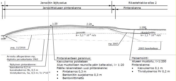
Figure 2. The initial plan was to use 0,20 m layer of moraine on top of tailings sand (on right the side of picture), which was substituted with 0,25 m fiber clay layer.
